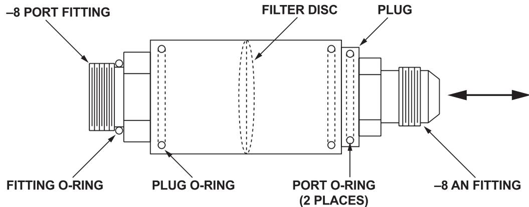
1. This filter is supplied with a 40 micron pleated stainless steel filter disc suitable for use as a pre-filter for Mallory fuel pumps or as a filter to protect carburetors.
