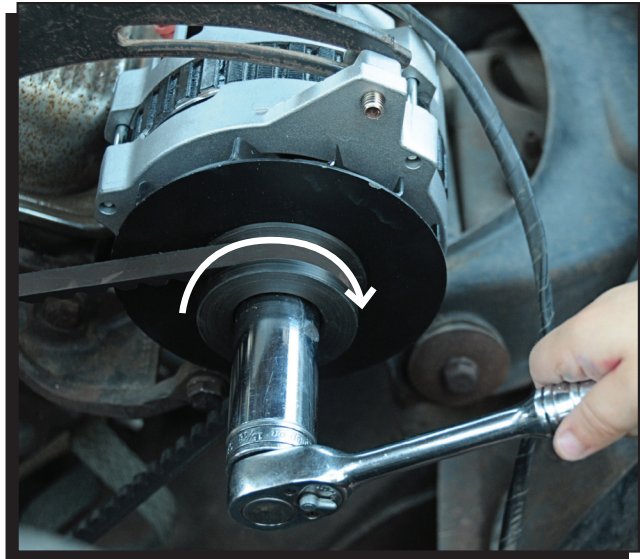
Figure 3 Checking Belt Tension.
