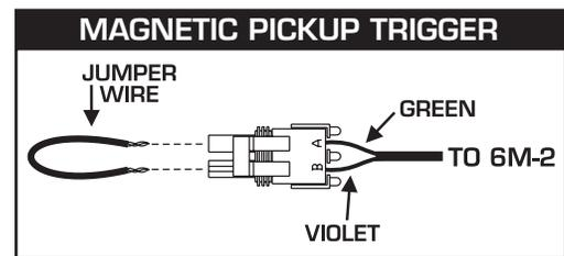
**Figure 8 Checking for Spark with Magnetic Pickup.**
