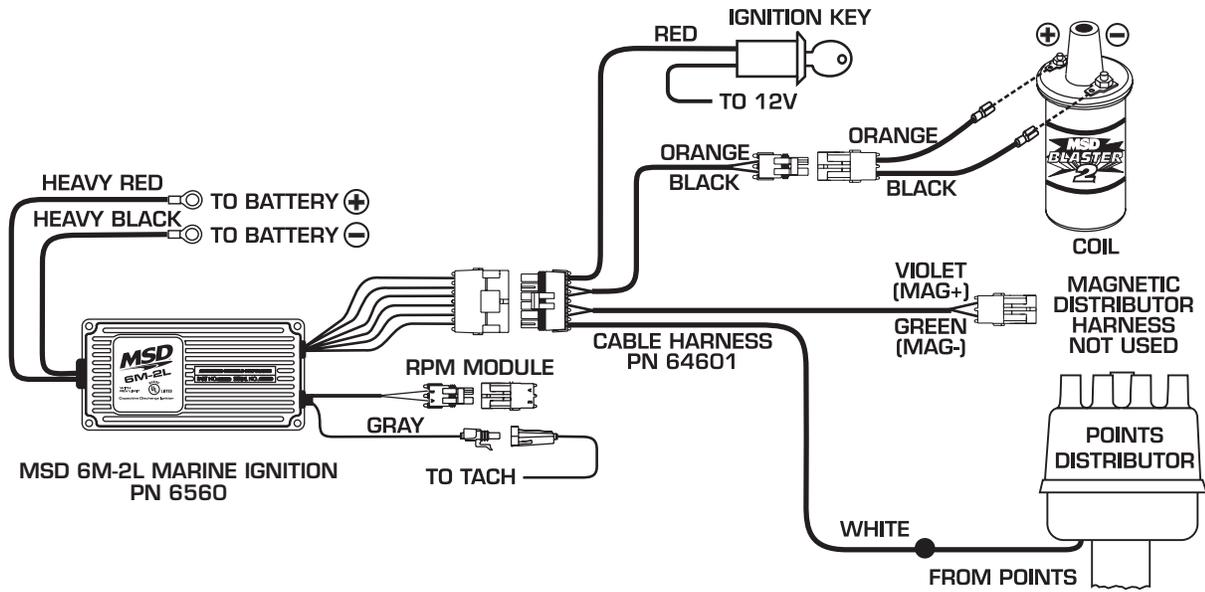
**MSD SYSTEMS MSD Marine Ignition to Magnetic Pickup Distributor**
