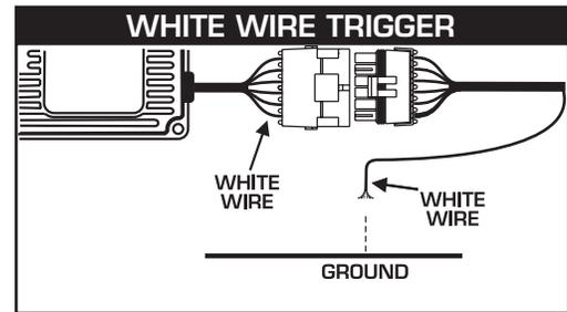
**Figure 7 Checking for Spark with the White Wire.**
