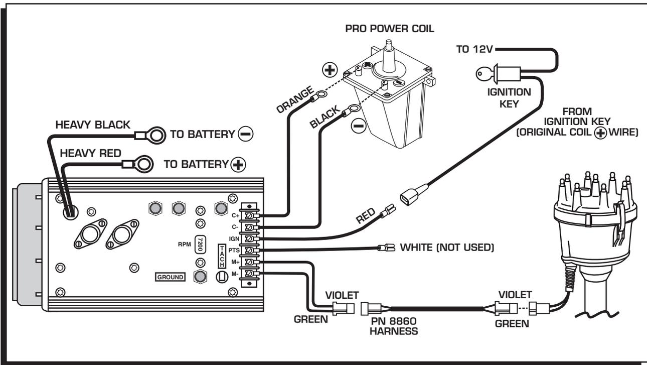
Figure 10 Wiring to an MSD 7-Series Ignition Control.
