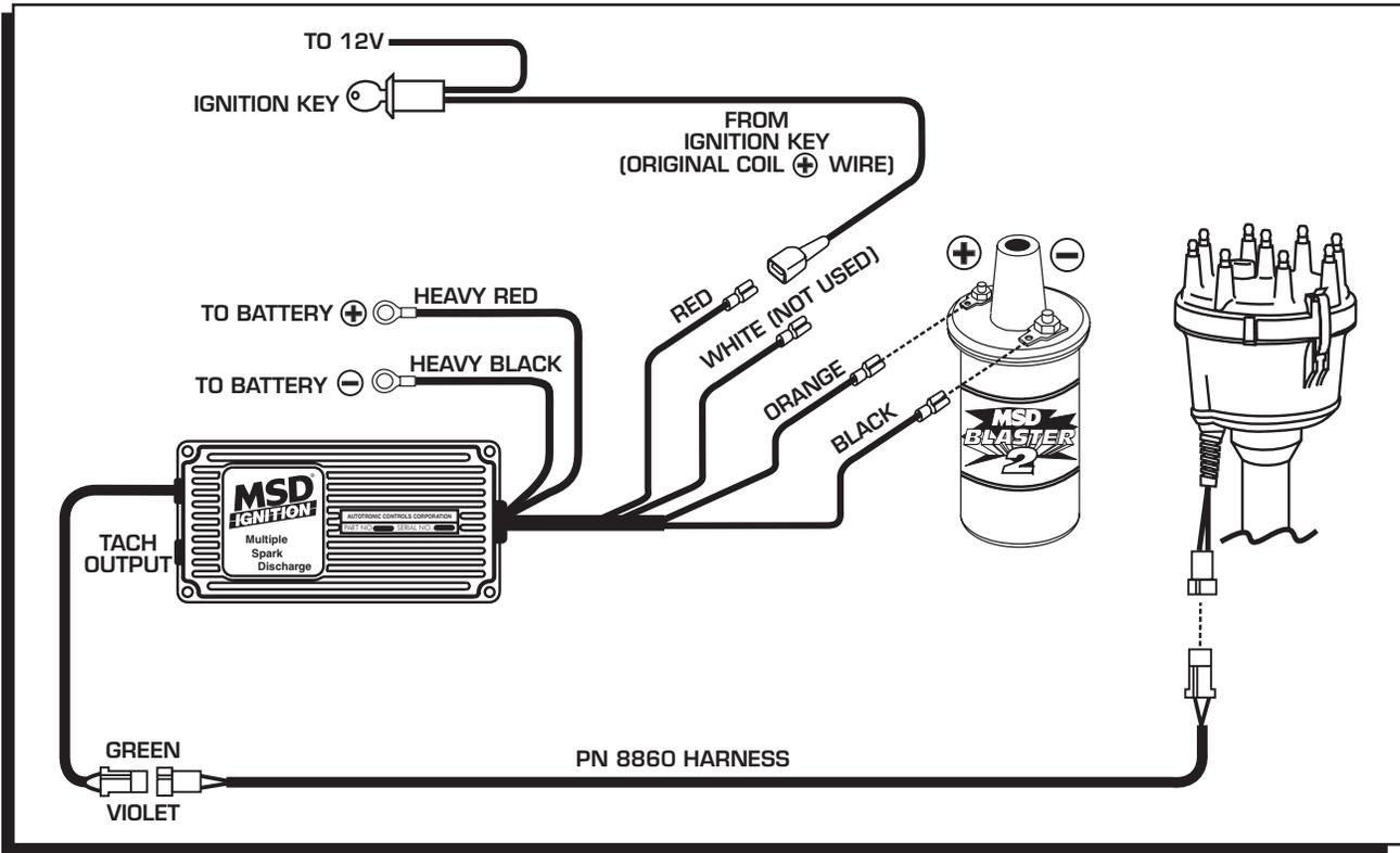
Figure 9 Wiring to an MSD 6-Series Ignition Control.
