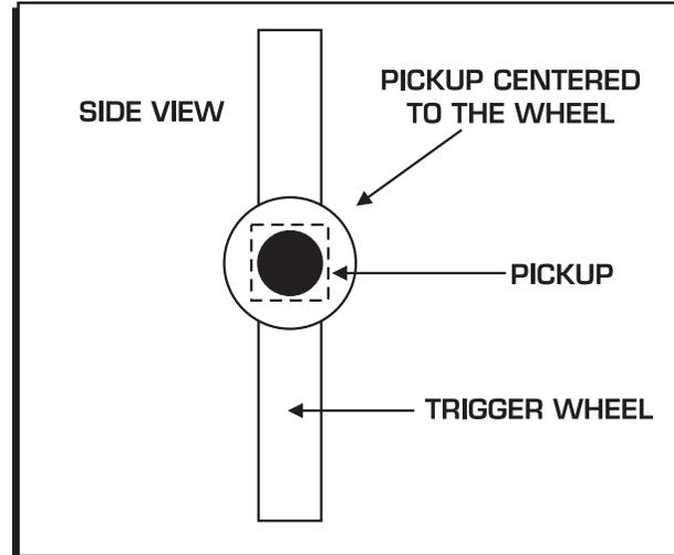
**Figure 2 Pickup Centered on the Trigger Wheel.**
