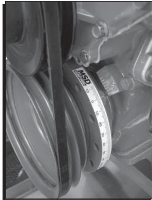
Figure 2 The Timing Tape Installed.
